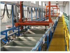
8. ELECTROPLATING Zinc plating Welded decking mesh -9 to 12 microns.
