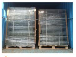
9. PACKING Finished products are placed on wooden pallet with angle boards on all sides and wrapped for safety of the product during transit.
