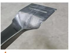
**O. STIFFENER FLATTENING** The stiffener from roll forming is then flattened on both sides based on reauirement.
