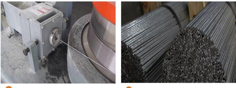
2. WIRE DRAWING PROCESS Higher dia wire rods are drawn to required dia.
