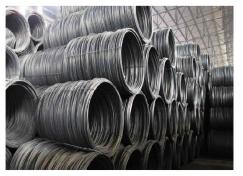
. WIRE ROD Low carbon wire rods are used for high quality welded wire mesh
