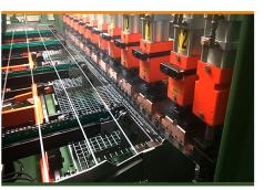
4. SPOT WELDING - 1 Pre-Cut wire rods are joined into mesh using spot welding at required temperture and pressure.
