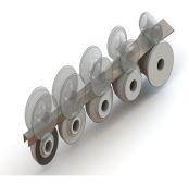
5. ROLL FORMING MS Coil of required width and thickness is used to make stiffener of required length.
